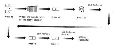
Note: Clear third limit point method and set the limit point;Long press the stop button for 2s, the blind moves to the third limit automatically;
