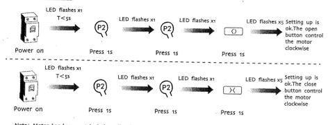
Note: Motor has been matched the code, don't use this method; Press the open button, if the curtain closed, please perform the reverse of direction setting.
